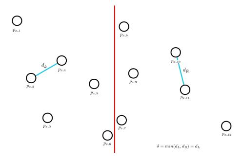
We need to determine if there are two points, one on each side of the dividing line, that have distance less than  $\delta$  from each other. We can eliminate all points that have distance more than  $\delta$  from the dividing line, since they cannot be less than  $\delta$  from any point on the other side of the line.
