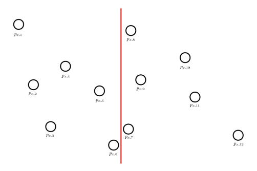
Fortunately we are able to avoid most of the potential computations. Let  $d_L$  be the minimum distance on the left side, and  $d_R$  be the minimum distance on the right side - we get these values from the recursive applications of the algorithm to the left and right halves of the set. Let  $\delta = \min(d_L, d_R)$ .
